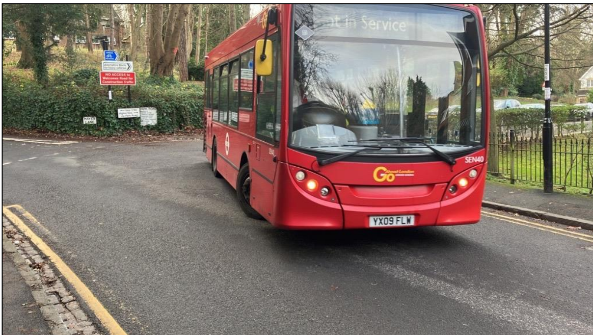
Figure 8: Image of the bus used on the test, having just made the turn from Park Road onto Hayes Lane (towards Whyteleafe). The driver has remained as close to the kerb as possible, but still cannot leave enough room for a vehicle to proceed in the opposite direction.
