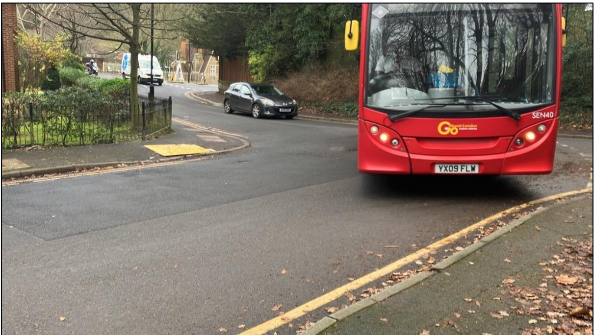
Figure 7: Image of the bus used on the test, having just made the turn from Hayes Lane onto Park Road (towards Coulsdon). There is more clearance to make this turn without infringing on the opposite lane, in this direction only.
